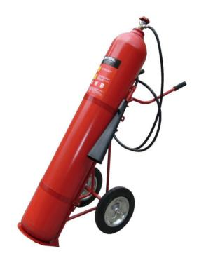
CO2 Extinguisher on Trolley is made of seamless cylinder to withstand the high storage pressure. It is effective on both Class B and C fires, and electrically non-conductive.
