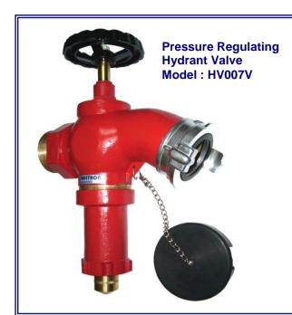
The **MULTRON** Pressure Regulating Hydrant Valve is self-regulating, that enables pressure to be maintained at any hydrant location in the system of a high rise building. Efficient pressure control is not affected by differences in inlet pressure, which may occur at varying floor levels. This self-regulating valve is very suitable for commercial buildings, oil refineries and chemical plants where varying high inlet pressure may also create problems.
