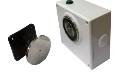
Model MD-111 Electromagnetic Door Holder are attractively styled and ruggedly constructed for easy and versatile installation. The contact plate can be adjusted to suit any door angle, with a holding force of approximately 35kg that can hold most types of doors.
