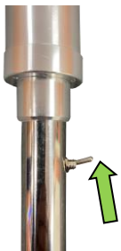
Smoke Detector Testing Position (Toggle Selector Switch Up )
